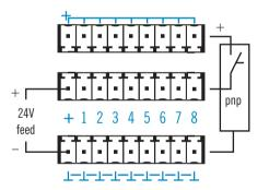
Caution! ground connections <100mA load (no busbar)
