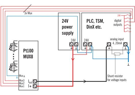
PT100MUX8 allows eight temperature sensors signals to be converted and multiplexed to a single analog output of 4..20mA. As such it is handy for temperature control using a standard PLC with few analog inputs or for ELZET80's controllers with analog voltage or current inputs. Except for an analog voltage input of 0..1 to 0..10V or a current input of 0/4..20mA, only three 24V digital outputs and a 24V/30mA supply are needed.
