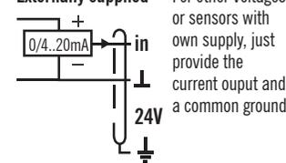
**Warning:** All 24V terminals are interconnected. Do not connect 24V to the jumpers. IS between 24V and 0V terminals is a common ground.
