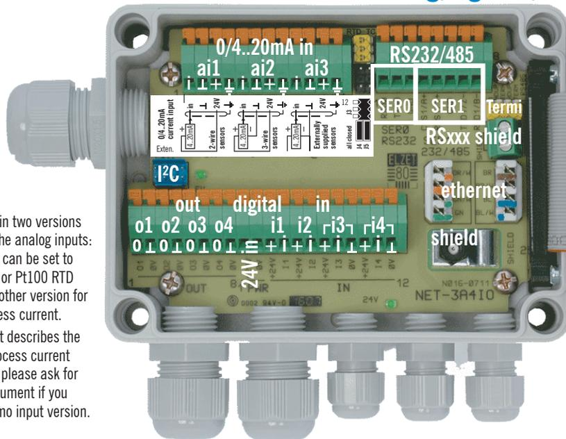
3A4IO comes in two versions that differ in the analog inputs: A version that can be set to thermocouple or Pt100 RTD inputs and another version for 4..20mA process current.
