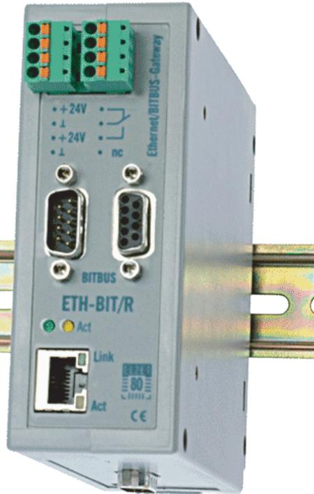
ETH-BIT/R is a rail-mount gateway between ETHERNET and BITBUS, working as master or as slave. It is based on the NET-A7S ARM processor board and comes with a firmware task that implements a BAPI-over-TCP-server (see [www.bitbus.org](http://www.bitbus.org)). The BAPI.dll software for Windows® emulates a local board for the PC and encapsulates BITBUS messages in TCP/IP messages to be sent to the BAPI/TCP server on ETH-BIT/R.
