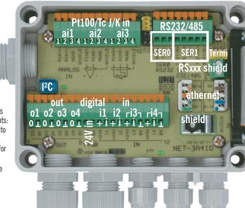
3A4IO comes in two versions that differ in the analog inputs: One version that can be set to thermocouple or Pt100 RTD inputs and another version for 4..20mA process current. This document describes the Pt100/Tc version. Please look/ask for the 3A4IO < I document if you have the 0/4..20mA input version.
